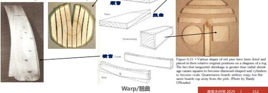
Figure 6.15 • Various shapes of red pine have been dried and placed in their relative original positions on a diagram of a log. The first flat tangential shrinkage is greater from radial shrinkage causes squares to become diamond-shaped and cylinders to become oval. Quarter-sawn boards seldom warp, but flat-sawn boards cup away from the pith. (Photo by Randy O'Rourke)
